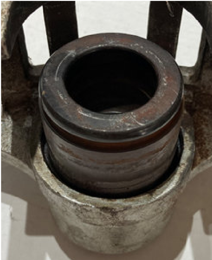
Figure 2. The swollen phenolic piston (Top). Note the scuff marks at the bottom of the piston caused when pumping out of the bore. The swollen piston will not slide into the bore (Bottom).
